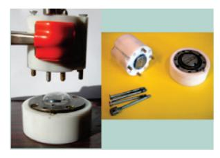
Figure 5. Electrochemical cell specially designed for pseudo in situ XRD study.
